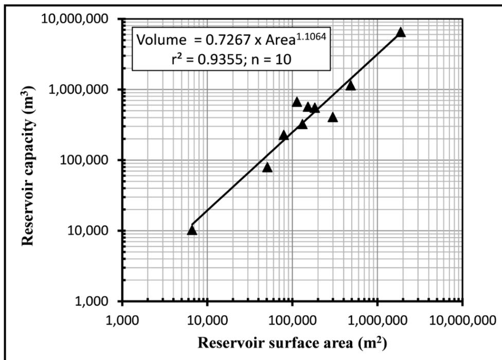
Figure 4. Power relationship between surface area and reservoir volume, Kaleya River basin.
