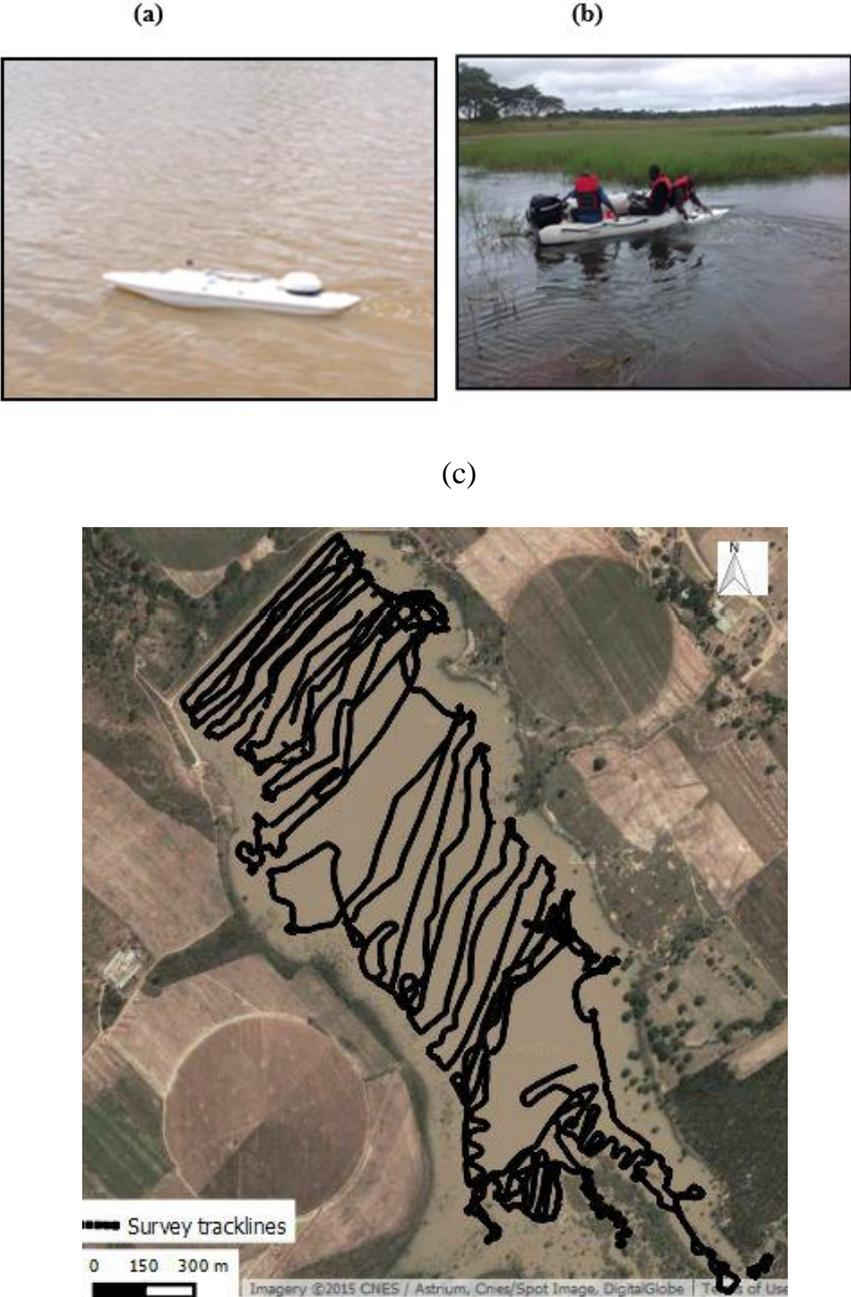
Figure 2. Coden Hydrographic boat (a) and motorized inflatable boat (b) used for dragging survey boat on reservoirs with weeds; and an overlay on Google image of survey path lines (c) showing the distribution of XYZ data points on Chisoba reservoir.
